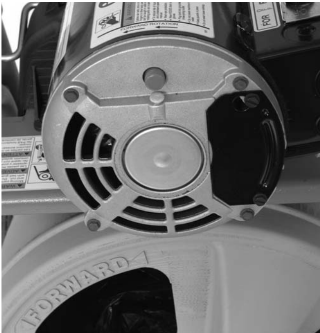
Figure 8 – Drum Rotation Direction Arrows
