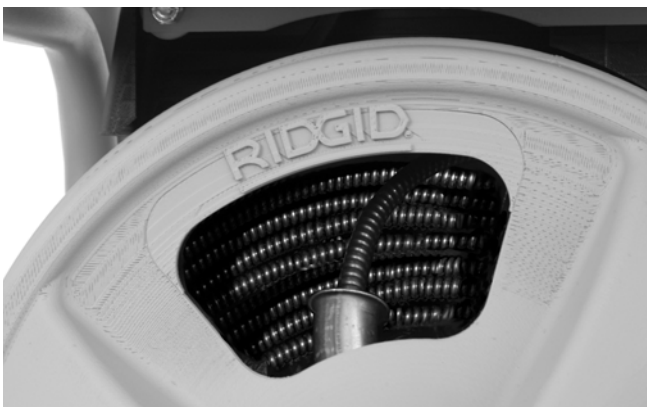
Figure 17 – Coil Cable Into Drum As Shown
