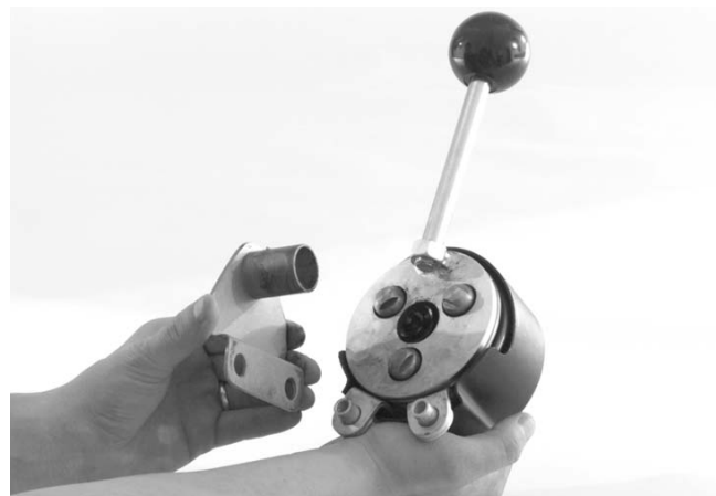
Figure 3 – Placing Mounting Bracket Into AUTOFEED
