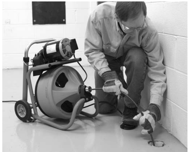
Figure 12 – In Operating Position, Manually Feeding Cable
