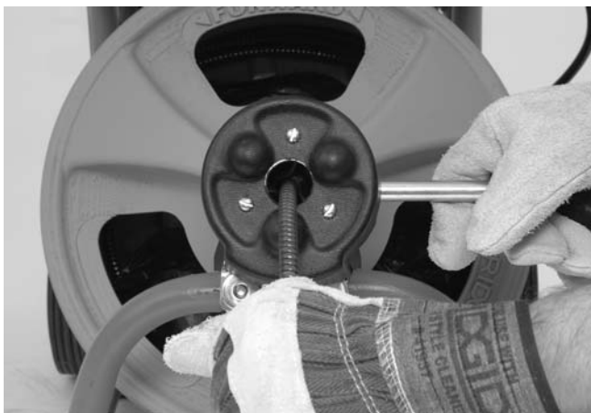
Figure 14 – AUTOFEED in Retrieve Position
