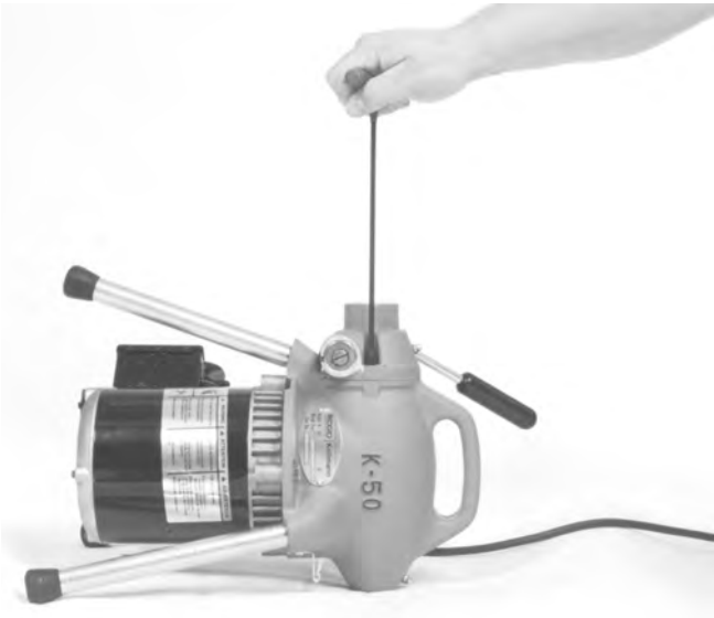
Figure 10 – Remove Socket Head Cap Screws
